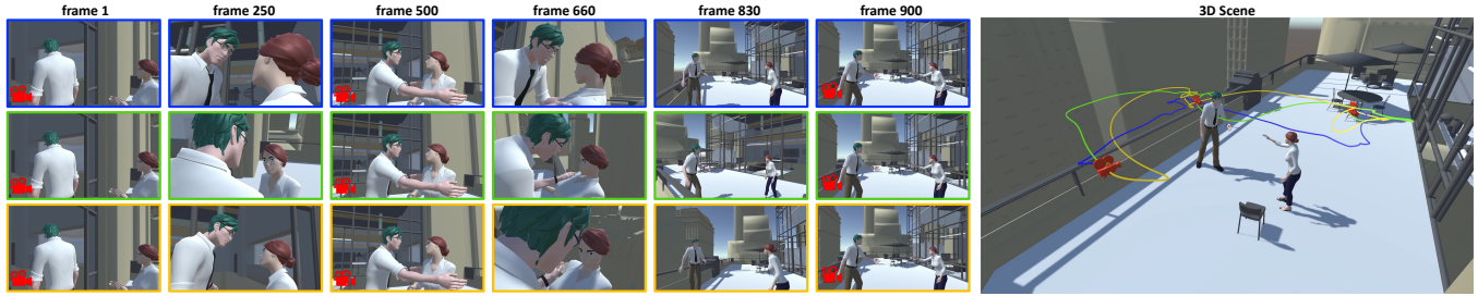
Fig. 10. Experiment with same keyframes and different behaviors: different colors represent different camera behaviors. Frames with red camera icon at the corner refer to keyframe constraints. We observe that constraints are well enforced in the 3D content and in the rendered snapshots.
